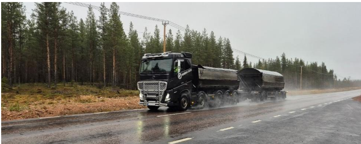
Picture 3-1: A Kaunis Iron truck has gross weight of 90 tons and a payload of 62 tonnes.
